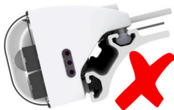
Mounted with beam too low.
