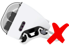
Mounted with beam too high.
