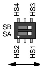
PTT Footswitch assignment can be set using SW1. The factory default is to assign input A to HEADSET 1 and input B to HEADSET 3.
