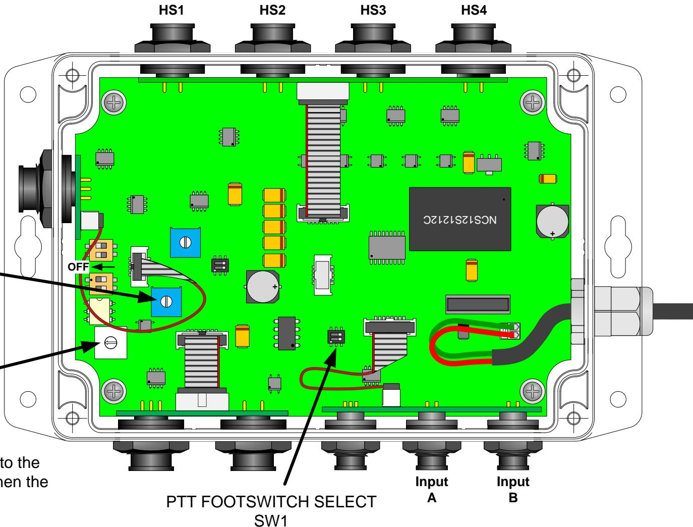
TX Audio level is normally factory-preset to the correct level for the radio type specified when the IM-977 is ordered.
