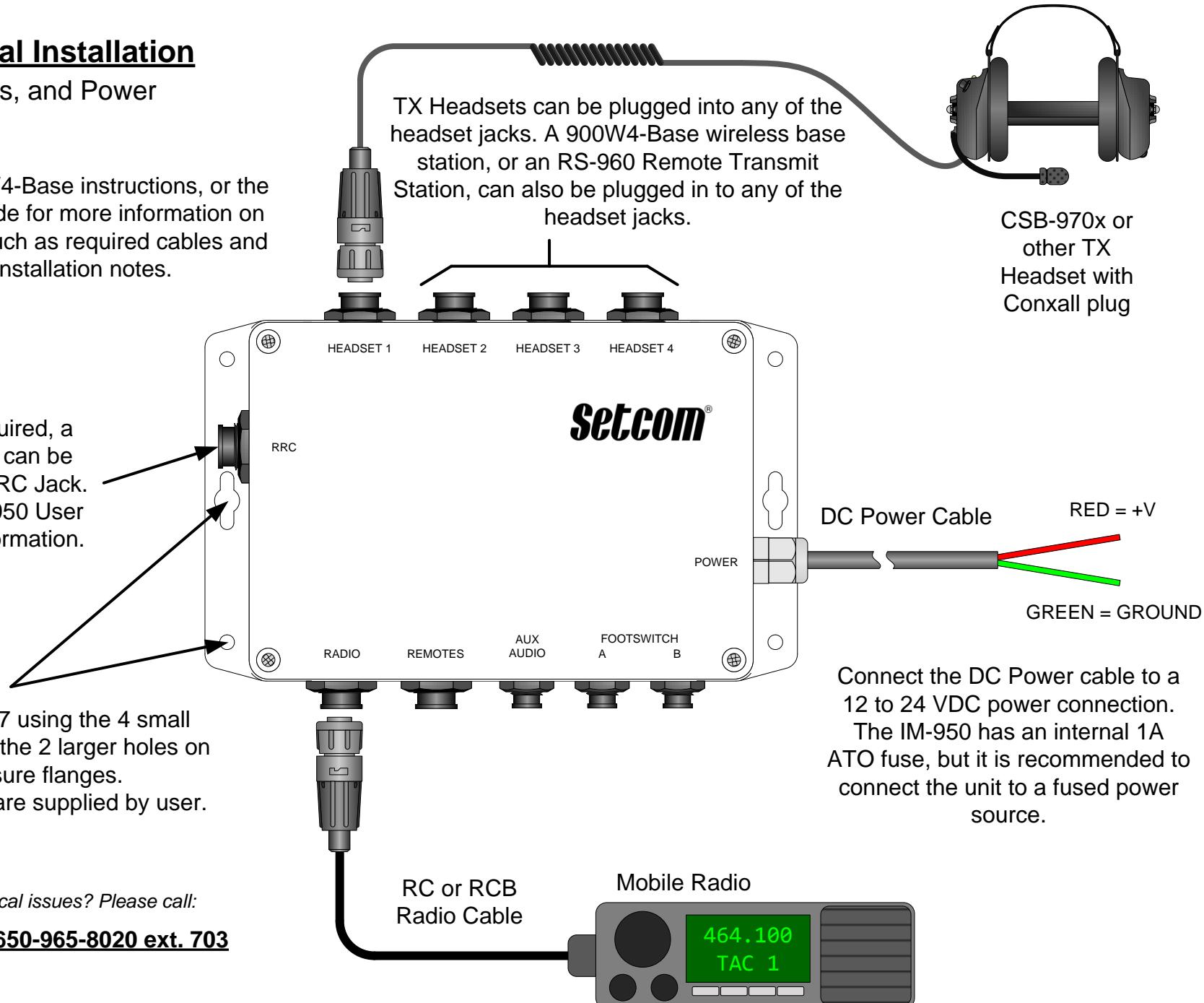
Radio Cable part number is determined by radio manufacturer, model number, and length of cable.
