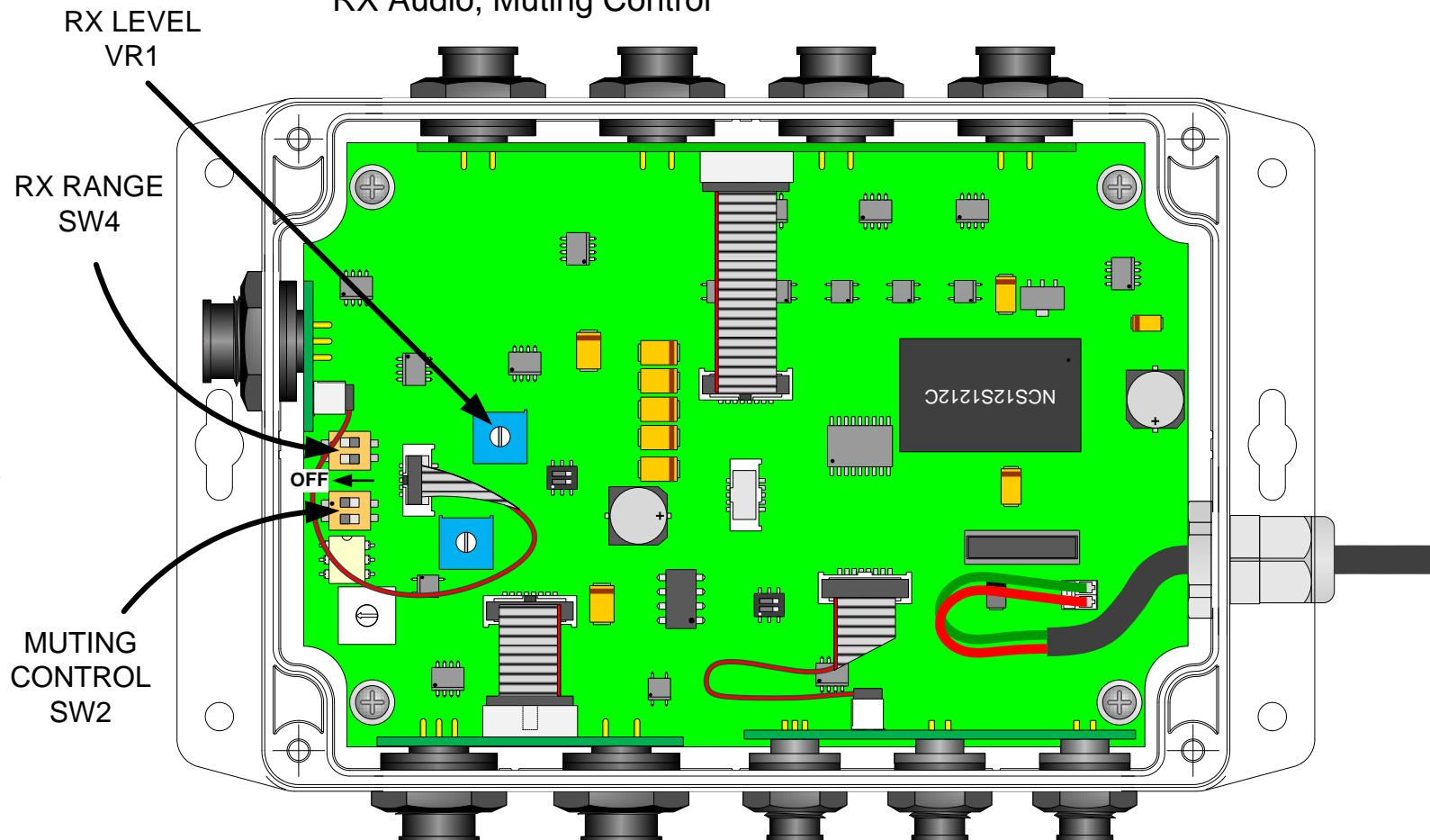
RX Audio level is normally set by the volume control on the mobile radio. If further adjustment is needed, RX LEVEL control VR1 can be used to adjust RX volume.
