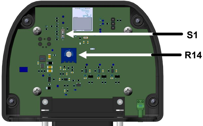
**Switch S1 is for PA Gain Adjustment, it is normally in the Off position. Setting it to the On position will increase the gain to the PA by about 9dB**
