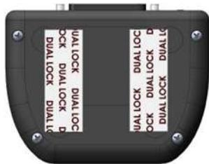
Once the selected area has been cleaned and dried, peel the two thin liners from the DUAL LOCK and place the MBT unit into position on the radio box LID.
